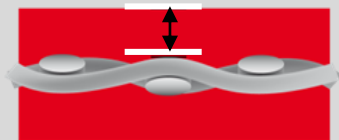
230 µm Serge Ferrari technology 650g/m 2
