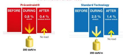
(Deformation test under load)
