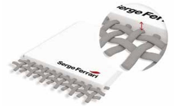
Serge Ferrari materials: coating of the high-strength polyester yarn membrane with layers of high performance polymers
